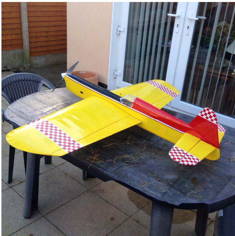
One of the most iconic of the FAI stunters in the 1960s The George Aldrich Nobler, powered by 35 Glow engines. Fox or OS 35s or even Merco 35s usually. This is a recent build (2015) from the old original 1960s Green Box Nobler Kit Electric Power!!
