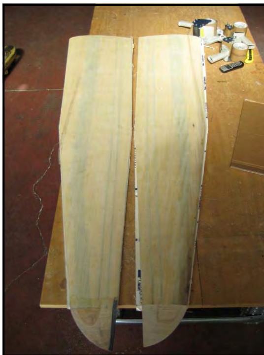
Wings completed: skinned with hardwood veneer.
