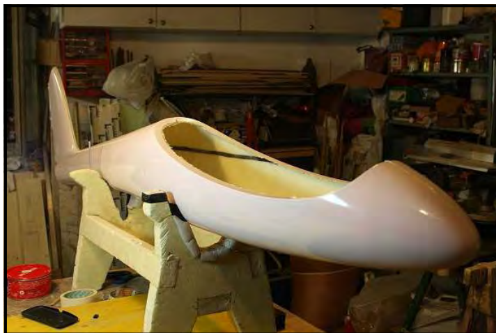
Complete fuselage out of the mould.
