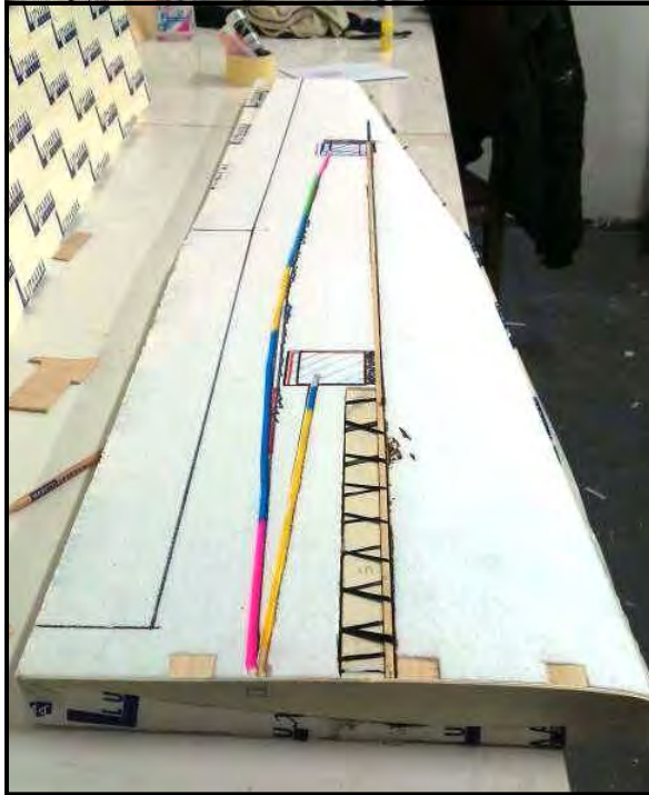
Wing core with main spar, joiner box and servo runs.
