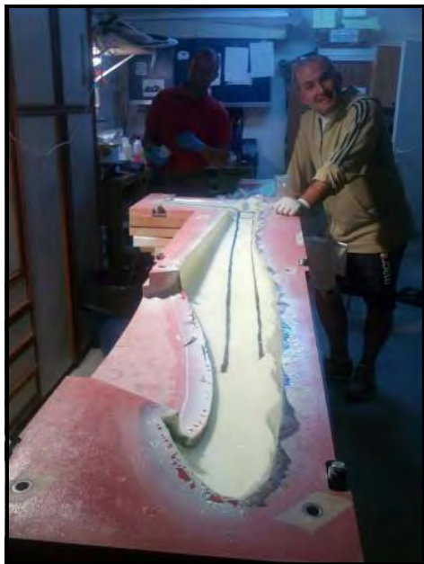
One half a fuselage in the mould.
