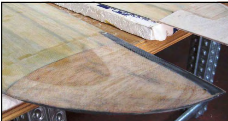
Wing tip with carbon reinforcing
