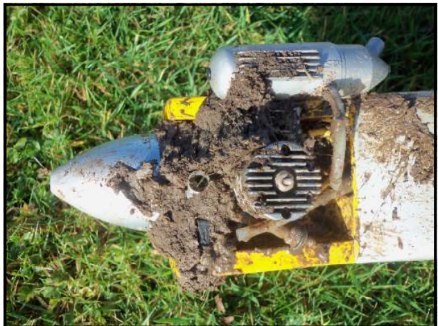
The O.S. 25FP after its near vertical full-throttle impact with the soggy, spongy ground. Engine has since been cleaned up, but not as yet test-run again.
