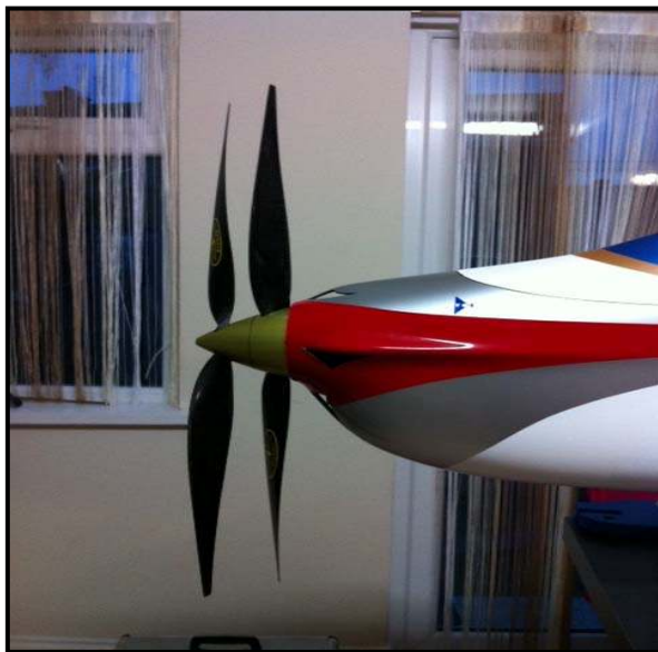
Front end of Gordon's machine an American Brenner set up running a 22 x 18 up first followed by a 22 x 20 behind this provides a very steady constant speed on the up and down lines.
