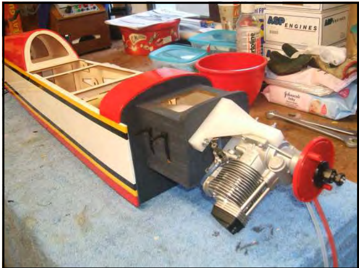
Edge 540 just after mounting OS 91 four stroke engine.
