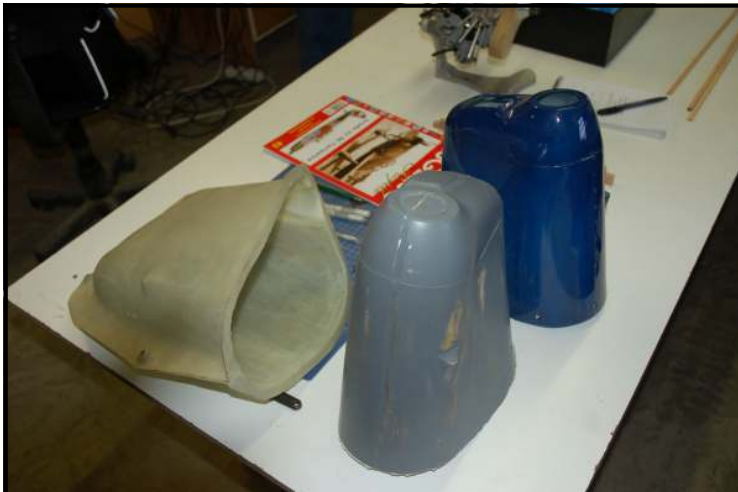
Cowl manufacture, shape, mould and final product.
