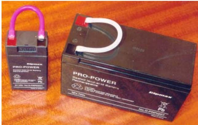
***Prevent possible gel-cell battery short-circuits by sheathing the terminals with silicone fuel tube.***
