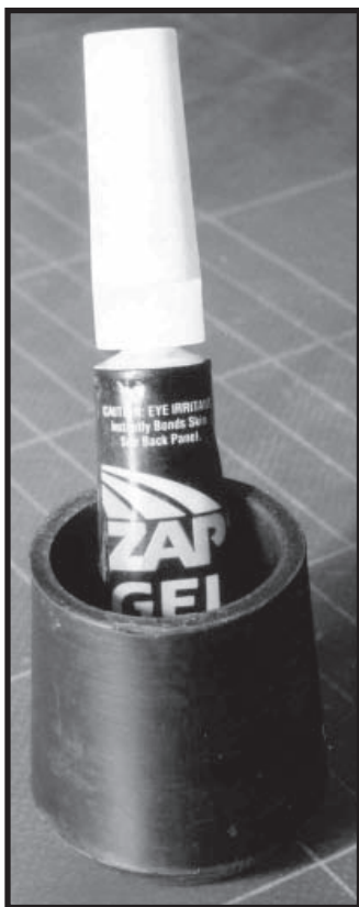
The rubber 'tip-sleeve' of a walking stick makes an ideal cyano tube holder.
